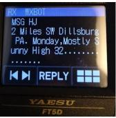
Some operators put their WX station data on APRS to send out current conditions as general APRS packets. They also show up on APRS.fi
