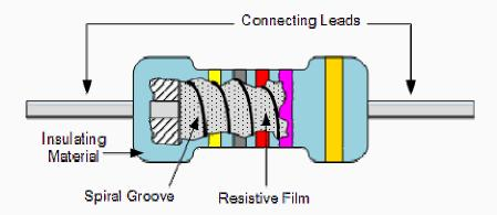
**Metal Film Resistors** have much better temperature stability than their carbon equivalents, lower noise and are generally better for high frequency or radio frequency applications. **Metal Oxide Resistors** have better high surge current capability with a much higher temperature rating than the equivalent metal film resistors.
