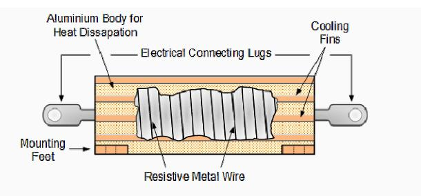
Wirewound resistor types are prefixed with a "WH" or "W" notation (eg WH10 $\Omega$ ) and are available in the WH aluminium cladded package ( $\pm$ 1%,  $\pm$ 2%,  $\pm$ 5% &  $\pm$ 10% tolerance) or the W vitreous enamelled package ( $\pm$ 1%,  $\pm$ 2% &  $\pm$ 5% tolerance) with power ratings from 1W to 300W or more.
