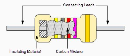
The **Carbon Composite Resistor** is a low to medium type power resistor which has a low inductance making them ideal for high frequency applications but they can also suffer from noise and stability when hot. Carbon composite resistors are generally prefixed with a "CR" notation (eg,  $CR10k\Omega$ ) and are available in E6 (  $\pm$  20% tolerance (accuracy)), E12 (  $\pm$  10% tolerance) and E24 (  $\pm$  5% tolerance) packages with power ratings from 0.125 or 1/4 of a Watt up to 5 Watts.
